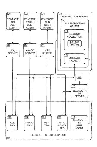
(57) Abstract: A system and method are presented in which a plurality of transport protocol objects (TPOs) (220, 221, 222, 223, 224, 225, 226 and 227) are instantiated at an IM user agent (115). In one embodiment, each of the plurality of TPOs (220, 221, 222, 223, 224, 225, 226, and 227) is adapted to provide a translation between a first IM protocol and a different IM protocol.
