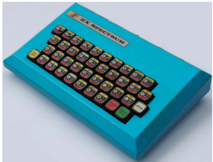
Figure 3. Spectrum-Contact, one of the variants of the Leningrad computer manufactured by the Leningrad-based start-up Taxuon [Tahion]. The computer was housed in a small, rudimentary plastic enclosure. The computer’s keyboard and its glossy stickers were readily available on the Speccy market and used in several other ZX-Spectrum clones. (Photograph by Z. Stachniak.)
