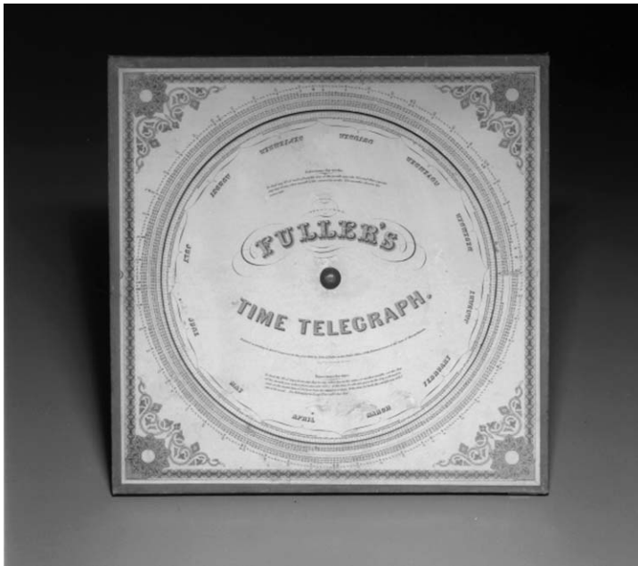
Figure 4. Fuller's Time Telegraph, London edition, 1860s. With Palmer's computing scale (a circular slide rule on the reverse side), this constituted Fuller's computing telegraph. (Smithsonian Institution, image number 87-4843.)
