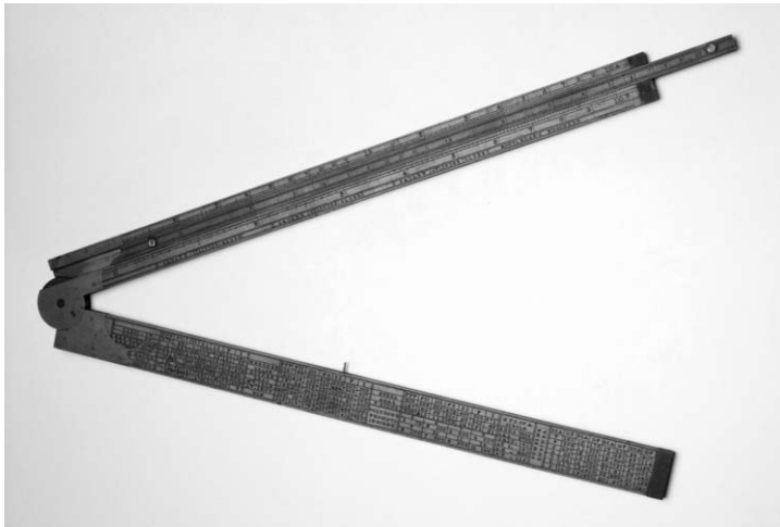
Figure 3. Routledge's Engineer's Rule by Thomas Aston of Birmingham, England, circa 1830. Such rules lack the girt line found on the carpenter's rule but have an additional logarithmic scale suited to calculations of squares and square roots, as well as appropriate tables to assist in calculations. (Smithsonian Institution, image number 82-6212.)
