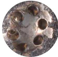
Injector after one P.i. treatment.
