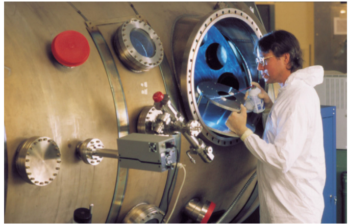
NIST staff using EUV reflectometer at NIST's SURF-III synchrotron facility to calibrate specialized optics for EUV lithography systems.
