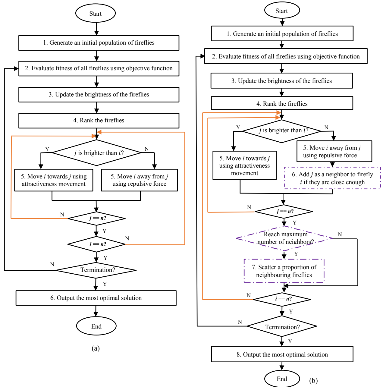
Figure 1 Flowcharts of the proposed two FA variants, i.e. (a) RFA and (b) SRFA
