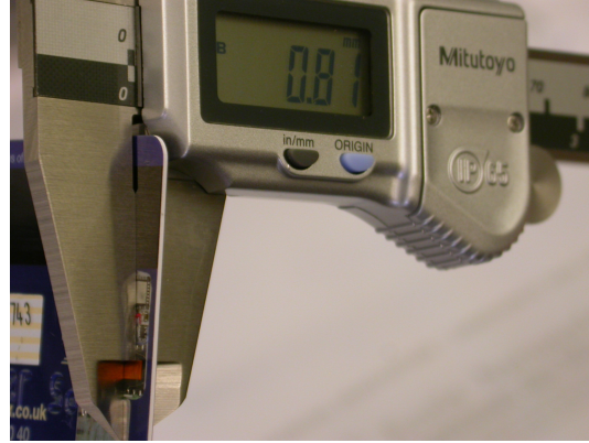
(b) Card is 0.8mm at thickest point so within tolerance for use within EMV terminals
