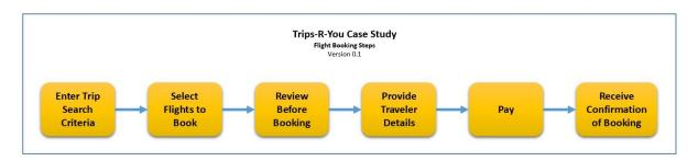
Detailed discussions about the UI supporting these steps were aided by hand-drawn screen mock-ups. There turned out to be a separate screen for each step shown above. In addition to the 'happy path' for the overall activity, alternate paths were identified. These involved the user wanting to modify
