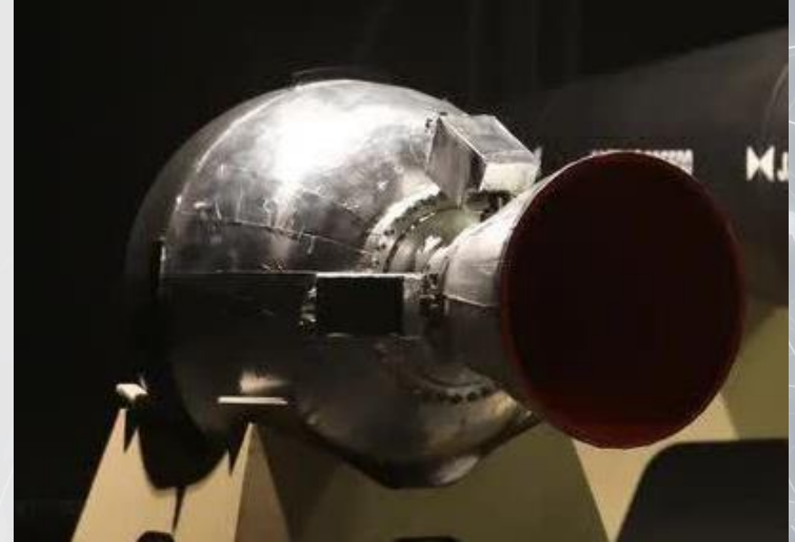
solid rocket motor hypersonic missile RV. Note the steerable nozzle .
