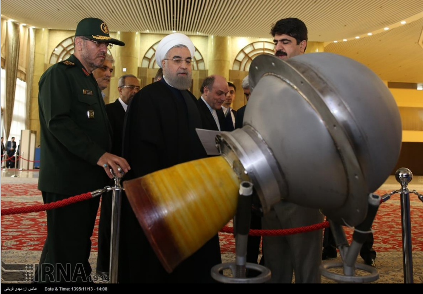
“Arash 24” solid rocket motor for space applications
