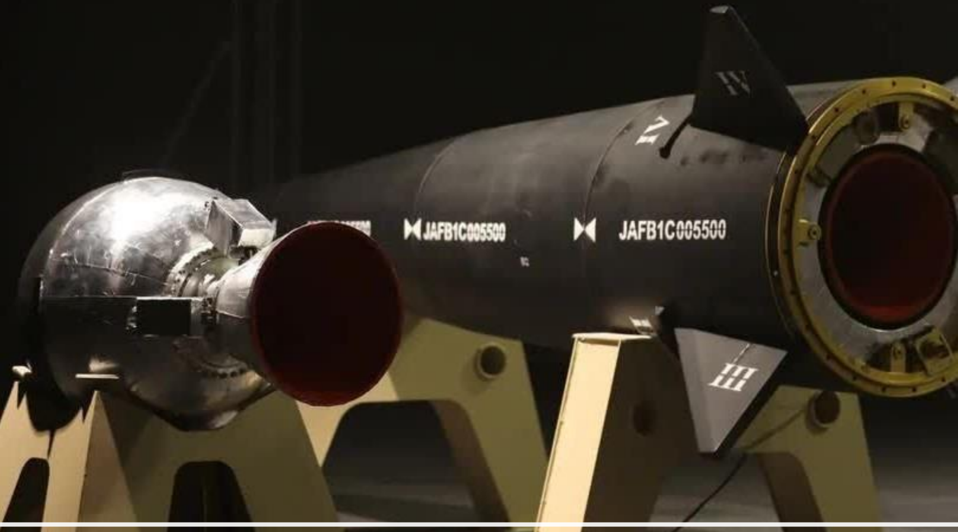
The “Arrash 24” solid rocket motor and the complete RV
