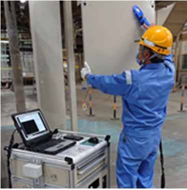
Surface coating image inspection equipment
