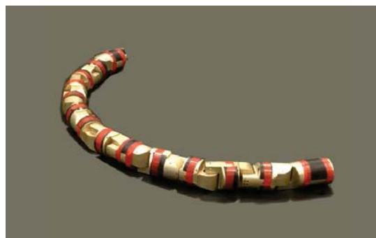
Fig. 1. The snake-like robot is rolling forward. This snake-like robot is modular designed. Each joint axis is orthogonal to its neighbors with a rotation range of \pm 90^\circ . Encoder and IMU sensors are mounted inside each module.
