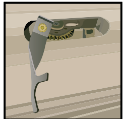
Construction Handle Tool may be used as a lock handle or crank handle.
