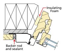
A. **Insert backer rod into the space around the window** so there is approximately 3/8" clearance between the backer rod and the exterior face of the window.
