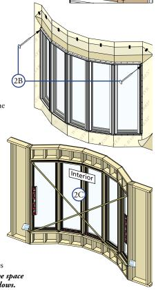
D. Check the interior reveal. Make sure the measurement from the interior face of the window to the interior face of the wall is equal at several points around the window.
