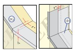
H. **Apply sill flashing tapes #2.** Starting with the flashing tape for one sill end, cut a piece 8" longer than the end unit width. Apply at the bottom of the opening so it extends 6" up the side, overlapping tape #1 by at least 1" and laps over approximately 1" onto the sill section for the next unit as shown. DO NOT allow the tape to extend past the interior face of the framing. Repeat this step for the other sill end.
