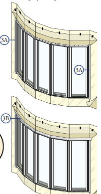
C. Fold down the top flap of the water resistive barrier.
