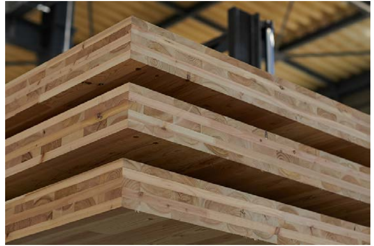
CLT manufactured at MEC Industry's own plant
