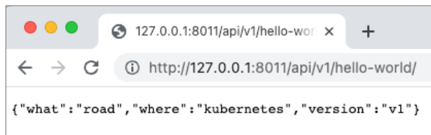
Figure 2.2 Uvicorn running FastAPI at port 8011
