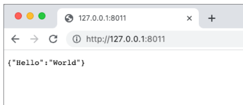
Figure 2.1 Uvicorn running FastAPI at port 8011
