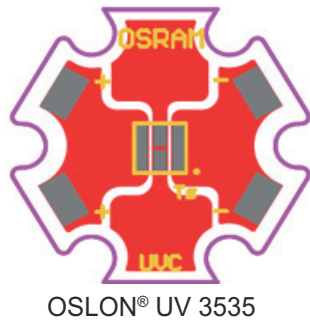
Figure 3: PCB layout of a single OSLON® UV LED on MCPCB
