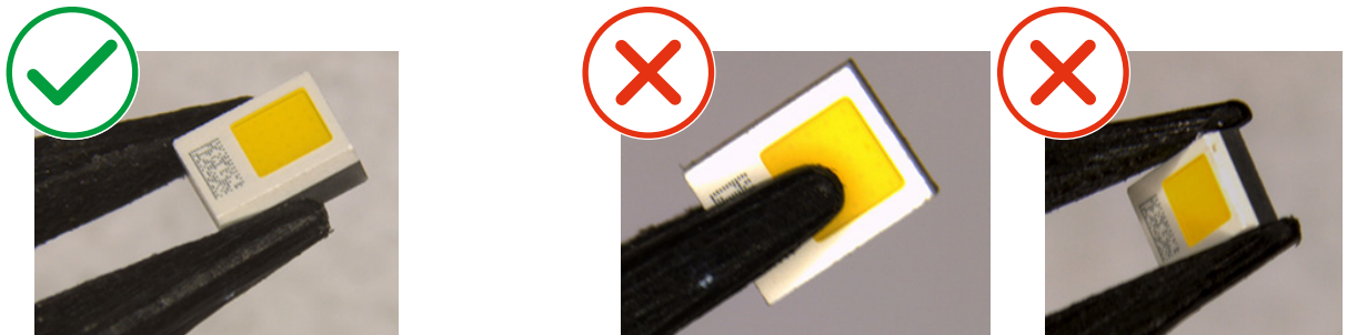
Figure 4: Correct handling on the ceramic substrate
