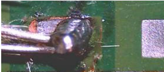
Figure 4: Attachment using high-temperature solder
