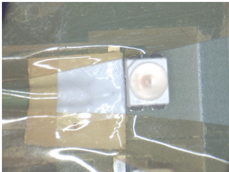
Figure 6: Example of temperature measurement on the solder pad of an LED, attachment with aluminum and polyimide tape
