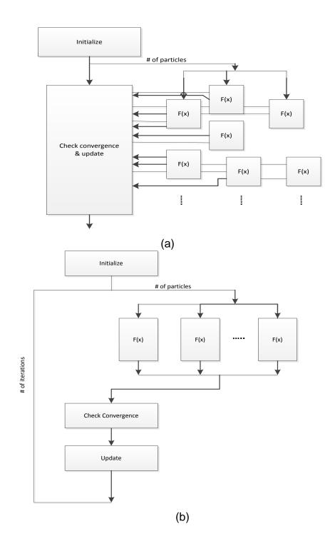
Figure 3.5: Block diagrams: (a) parallel asynchronous; (b) parallel synchronous PSO
