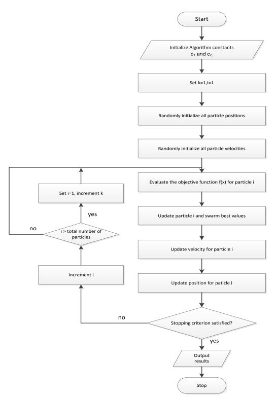
Figure 1.1: Serial implementation of PSO algorithm
