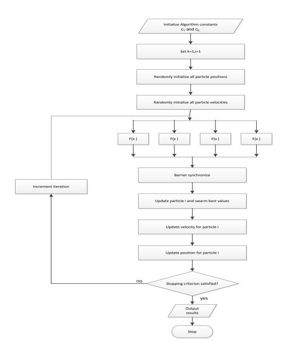
Figure 3.4: Parallel implementation of PSO algorithm
