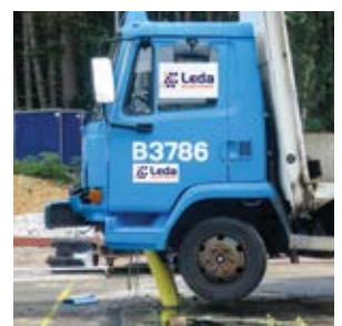
Above, 2500kg, 3500kg and 7500kg vehicle crash tests. Leda is the only Australian bollard manufacturer to have undertaken government-endorsed impact testing using different vehicle weights at various speeds.
