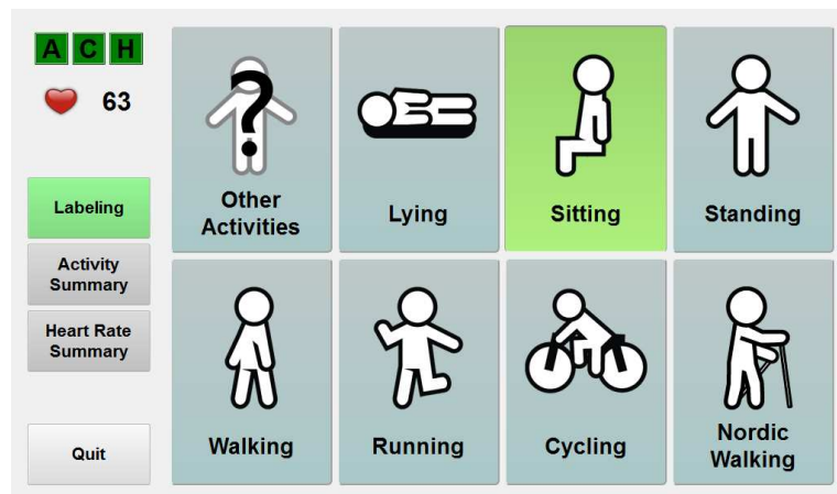
Figure 3.2: PAMAP2 dataset, GUI used for the data collection: start screen of the labeling tool. This screenshot is made while the subject is performing the activity sit during data collection. All sensors are operating correctly according to the green symbols in the top left corner. Moreover, the subject’s heart rate is 63 beats per minute in the moment of this screenshot, as indicated in the top left corner as well.
