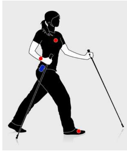
Figure 3.1: PAMAP dataset: placement of IMUs (red dots) and the data collection unit (blue rectangle).
