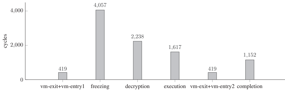
Fig. 12. Execution times of the steps in the in-place execution method (in which the preemption timer was set to 16). The columns represent the following steps (from left to right): entering and exiting the host; decrypting the function; executing the function; entering and exiting the host; erasing the decrypted function.
