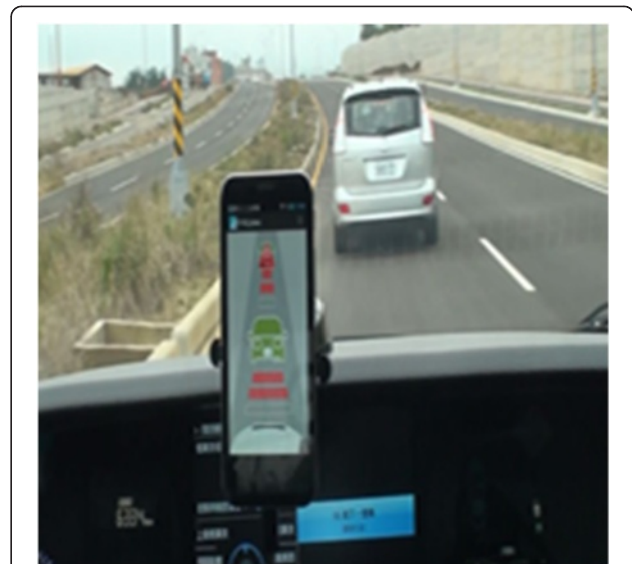
Figure 14 Emergency braking warning system in the same lane.
