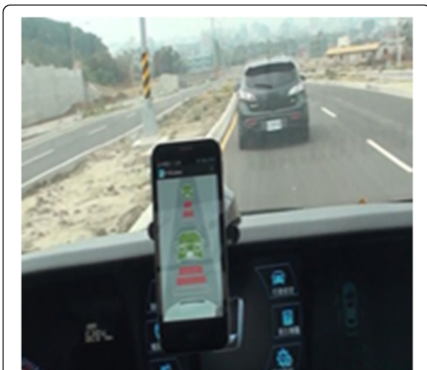
Figure 13 Communication-based forward collision warning.
