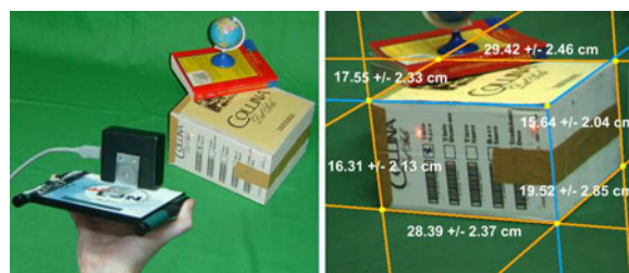
Figure 1. Scanner prototype: (left) Its operation. (right) Camera's view from another position showing the recovered dimensions and uncertainty computed in real time.
