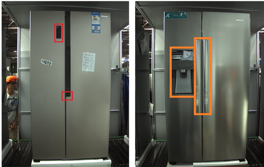
Fig. 3 The large homogenous areas and subtle salient regions in the front-view images of refrigerator
