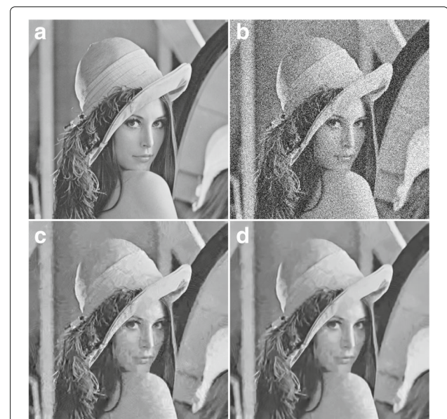
Fig. 4 Subjective assessment between the normal profile of BM3D and the proposed method. a Original image. b Noisy image at noise level \sigma = 50 , PSNR = 14.60 and SSIM = 0.1163 . c Output using the normal profile of BM3D, PSNR = 28.29 and SSIM = 0.7455 . d Output using the proposed method, PSNR = 28.97 and SSIM = 0.7972
