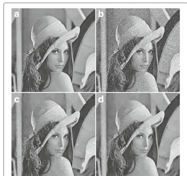
Fig. 5 Subjective assessment between the fast profile of BM3D and the proposed method. a Original image. b Noisy image at noise level \sigma = 50 , PSNR = 14.60 , and SSIM = 0.1163 . c Output using the normal profile of BM3D, PSNR = 28.28 and SSIM = 0.7438 . d Output using the proposed method, PSNR = 28.93 and SSIM = 0.7967
