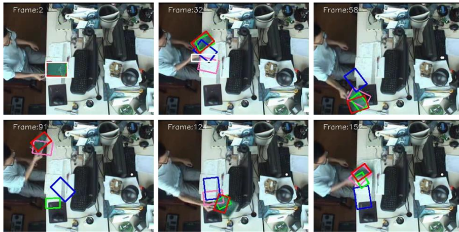
Fig. 13 The tracking results for the video “book” using CAM-Shift (white), PF (blue), VAPF (green), M-PF (pink), and the proposed tracker (red). Particle number N = 300
