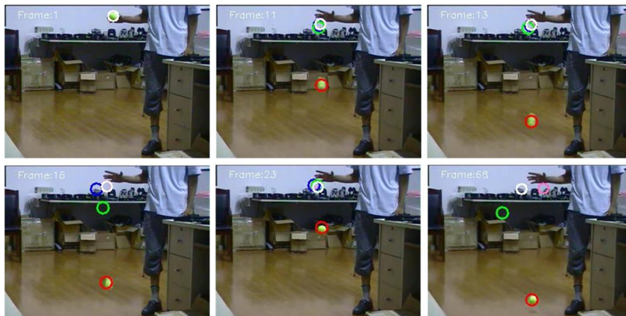
Fig. 16 The tracking results for the video “tennis” using CAM-Shift (white), PF (blue), VAPF (green), M-PF (pink), and the proposed tracker (red). Particle number N = 200
