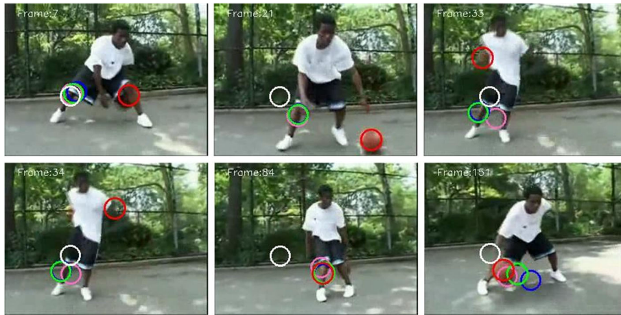
Fig. 15 The tracking results for the video “basketball_2” using CAM-Shift (white), PF (blue), VAPF (green), M-PF (pink), and the proposed tracker (red). Particle number N = 250
