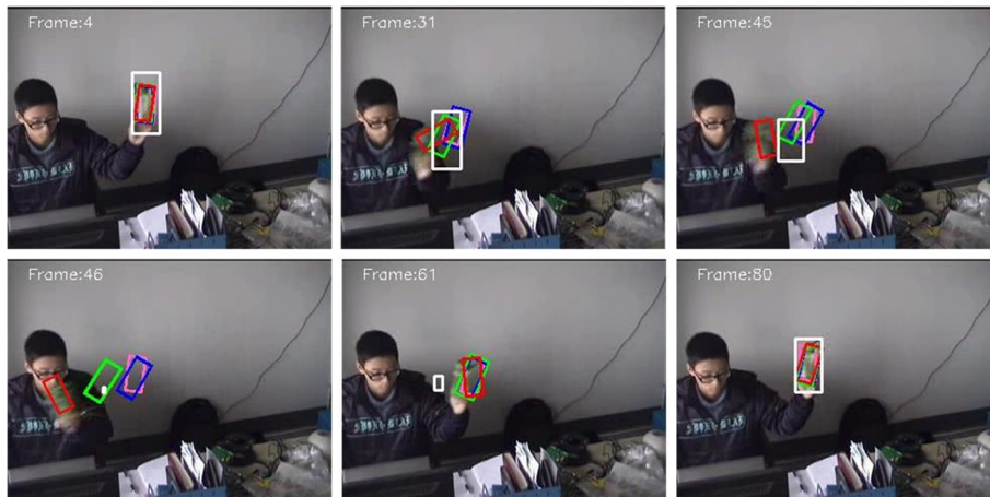
Fig. 12 The tracking results for the video “bottle” using CAM-Shift (white), PF (blue), VAPF (green), M-PF (pink), and the proposed tracker (red). Particle number N = 200
