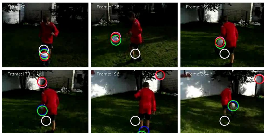
Fig. 27 The tracking failure example of video “v_juggle_15_02” using CAM-Shift (white), PF (blue), VAPF (green), M-PF (pink), and the proposed tracker (red). Particle number N = 250
