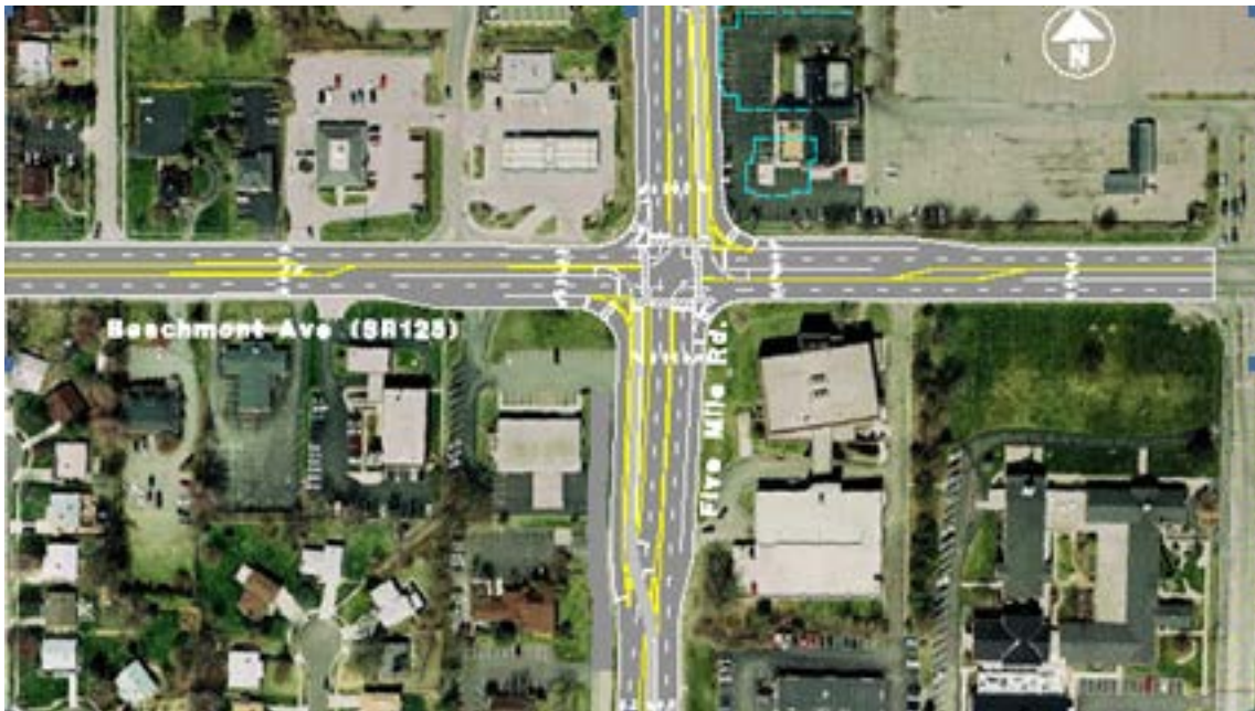
Figure 9-3: Five Mile Road Partial Continuous Flow Intersection
