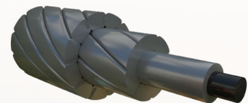
Figure A-101. TS conductor.
