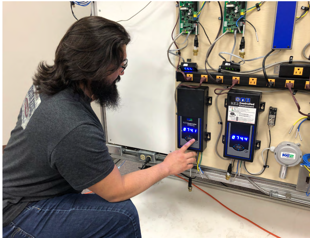
The KE2 Evaporator Efficiency controller provides energy savings of 15-50% compared to mechanically controlled systems.
