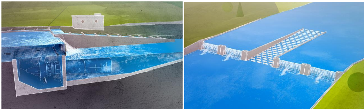
Figure 1: Simple, single shaft powerplant (left) and multi-shaft power plant with eco-migration corridor (right). (Th. Kaufmann/TUM)
