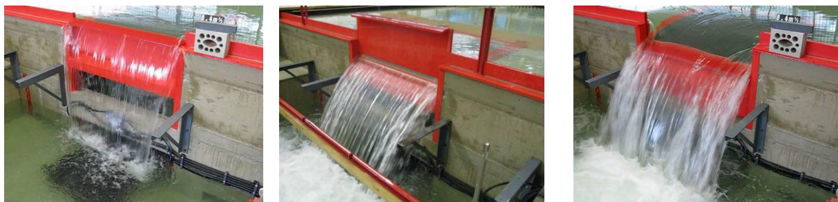
Fig. 4: Operating states: KW-operation (l.), Rack cleaning (m.) Bed-load and HW flushing (r.)
