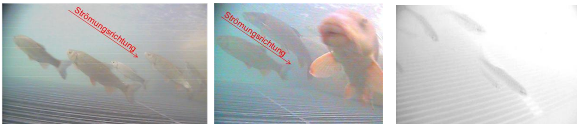
Fig. 8: Fish movement over the horizontal rack plane (l. chub, m. barbe, r. juveniles)
