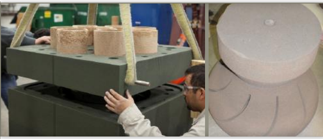
Manufacture 3D Printed Sand Mold & Cores and Assembly of Molds
