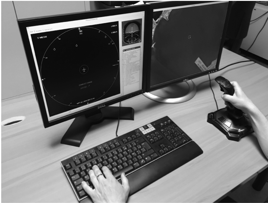
FIGURE VI.1 – Schematic Representation of the Apparatus during the Experiment. The Supervision task is displayed on the left screen and the Tracking task on the right screen.
