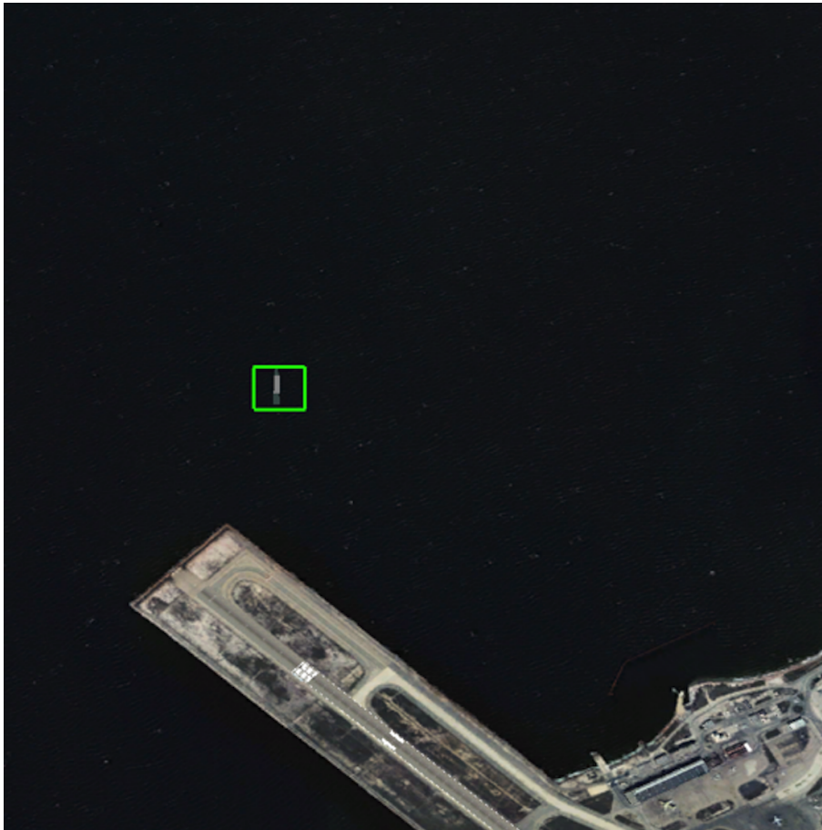
FIGURE VI.3 – Representation of the target and the cursor. If the coverage is higher than 75% of the target's surface, the cursor appears in green otherwise it appears in red.
