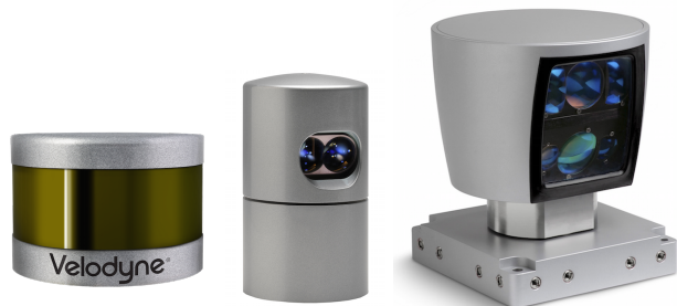
Fig. 2 From left to right: VLP-16, HDL-32E, and HDL-64E high-definition range scanners manufactured by Velodyne. These rotating scanners feature a complete 360° horizontal field of view as well as 16, 32 and 64 laser-detector pairs spread over a vertical field of view. The sensors range is from 1 m and up to 120 m (depending on the material properties of the scanned object) with a accuracy of 2 cm.
