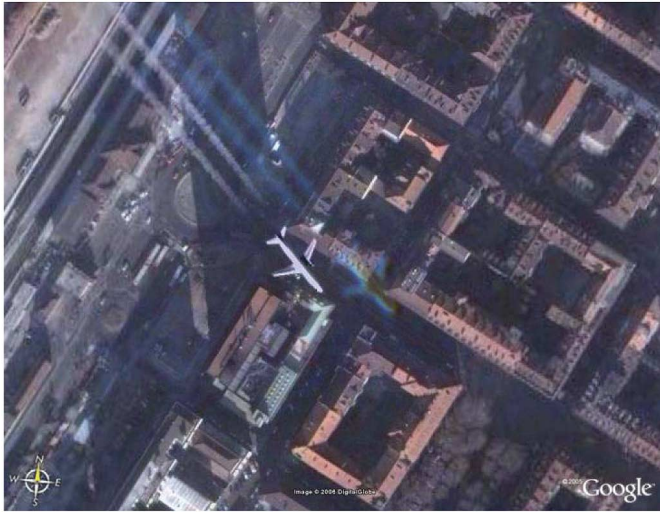
Fig. 5. True-color composition of fused Quickbird images (0.7 m) extracted from Google Earth over the city of Turin, Italy. Illustration of the default of ghost caused by fast-moving objects. Copyright Google.
