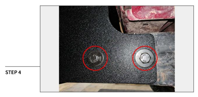
Install the new bumper to frame rails using the (2) M12 x 40mm bolts, flat washers, and lock washers. Torque to 40 ft. lbs.
