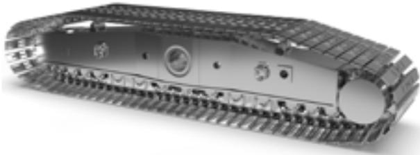
**Side frames B12** size for a giant bucket wheel excavator of 850 t machine weight. ITM supplies tailored components to optimise performance and reliability.
