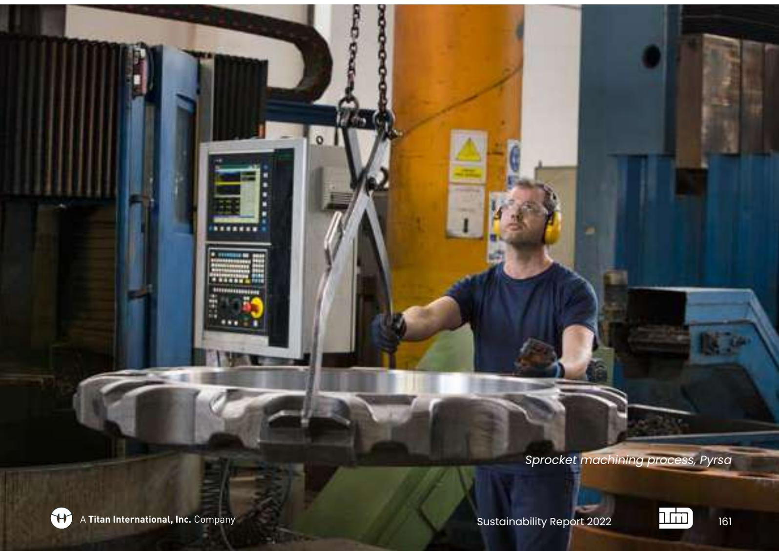
*Sprocket machining process, Pyrsa*
