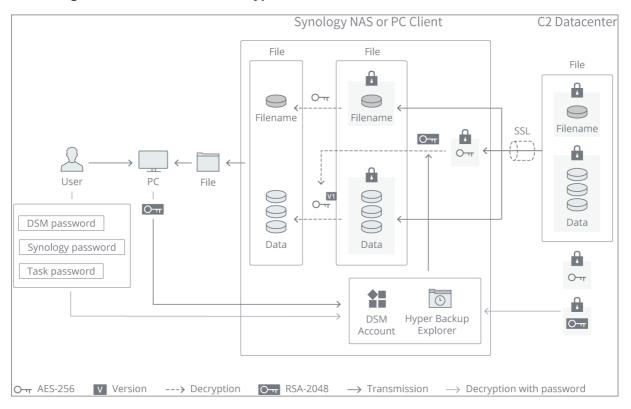
Figure 4: Users are advised to store RSA private keys to a personal device. Importing RSA keys to Hyper Backup Explorer or Synology NAS is the recommended way to decrypt files. However, users can also unlock RSA keys with a password set separately for each task.
