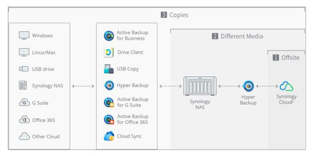
Figure 1: Synology provides a host of methods to back up data to Synology NAS. To protect against local disaster, cyberattacks, or IT failure, remote copies of backups can be stored to the cloud with C2 Storage, completing a "3-2-1 backup strategy."
