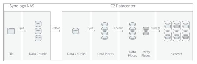
Figure 3: Data uploaded to C2 servers are split into pieces and encoded, generating parity pieces that keep data retrievable when one ore more servers are down.
