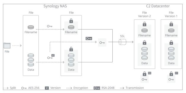
Figure 2: AES-256 client-side encryption of data chunks yields an AES key, which is encrypted with RSA-2048 and stored on the server. Cloud storage providers are not only expected to prevent unauthorized access to private files, but also to guarantee that data are continuously available and remain in top shape over long periods of time.
