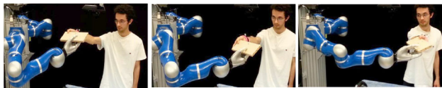
Fig. 12 Handover of a plate. Conditioning on three different positions of the wrist (using motion capture) of a human coworker
