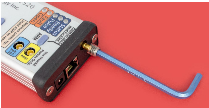
Figure 13: Removing blanking plug.
