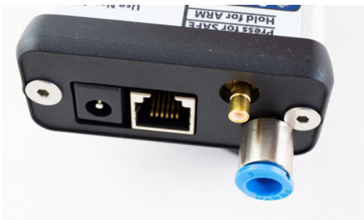
Figure 14: Adding air inlet adapter.
