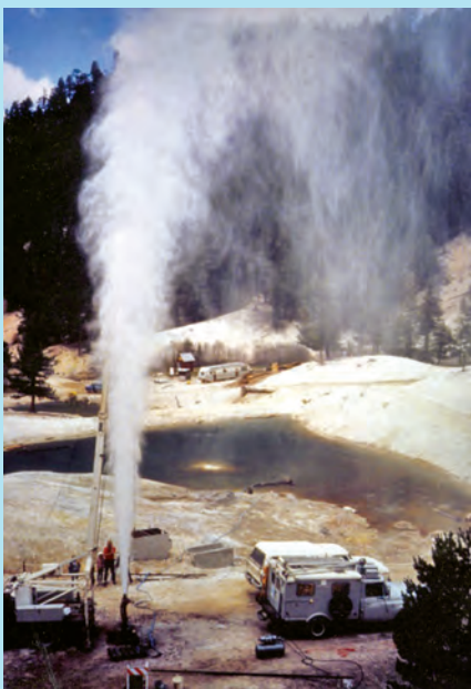
Flow test of well VC-2a, May 1987, Sulphur Springs, Valles caldera, from a single fracture in Bandelier Tuff at 1,607 feet, 410° F. The geothermal "reservoir" underlies a thin cap of acid hot springs, fumaroles, and gas vents surrounded by rocks containing sulfur, kaolin, and other acid-stable minerals. Author photo.
