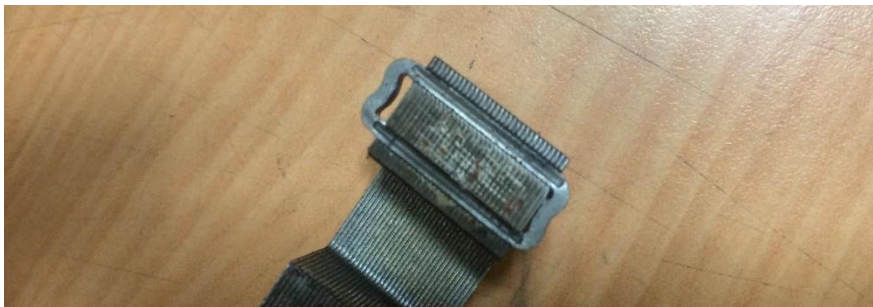
Figure 2.23: Deteriorated shading rings
