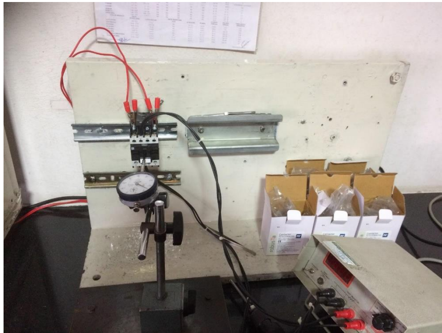
Figure 3.1: Travel Gauge setup for Overtravel and Total Travel Calculation
