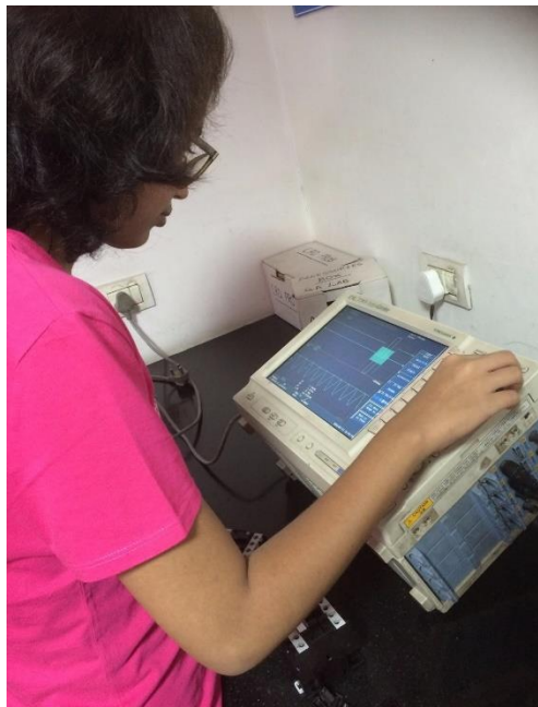
Figure 3.31: Observing and Measuring the Closing and the Opening Time using CRO Oscilloscope
