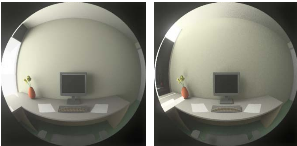
Figure 7. Each window pane contributes independently to the amount of light present in the room. For June 12th at 1 PM standard time, the image on the left shows the contribution of the lower pane, the one on the right the contribution of the upper pane.
