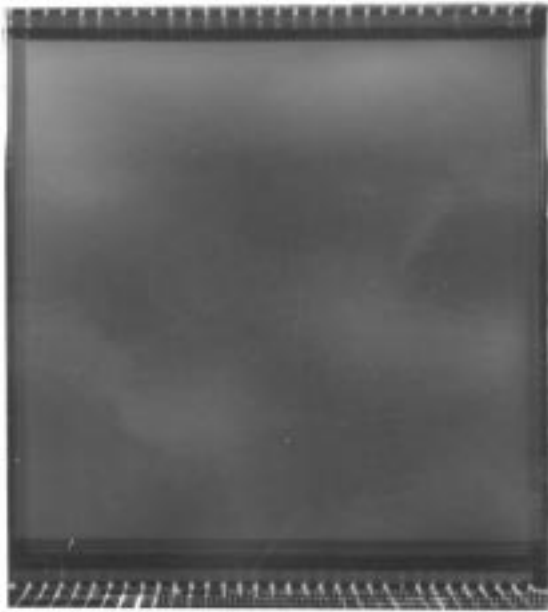
Fig. 8. 1024 \times 1024 element photogate CMOS APS with 10\text{-}\mu\text{m} pixel pitch fabricated using 0.5\text{-}\mu\text{m} design rules by AT&T/JPL.
