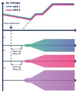
Dc voltage and AC current behaviour using the same value for delay time
