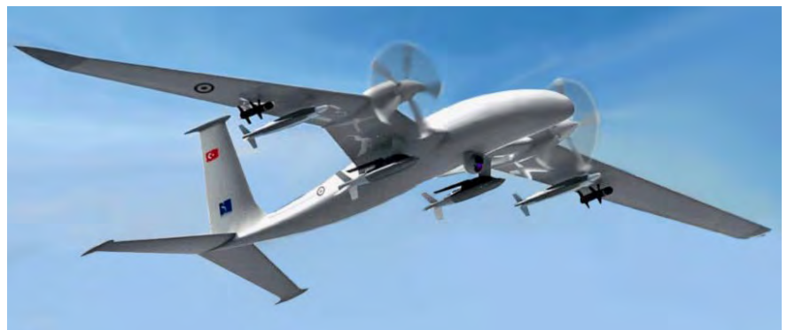
The high-altitude, long-endurance Akinci drone can stay airborne for more than 24 hours. / Ukrainian defence ministry, cc-by-sa 4.0
