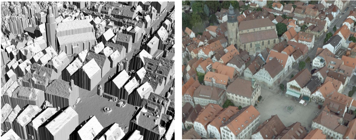
Figure 5: Automatic untextured and textured reconstruction from DGPF UltraCam-X images with 8 cm/pixel ground sampling distance (from Hirschmüller and Bucher, 2010).
