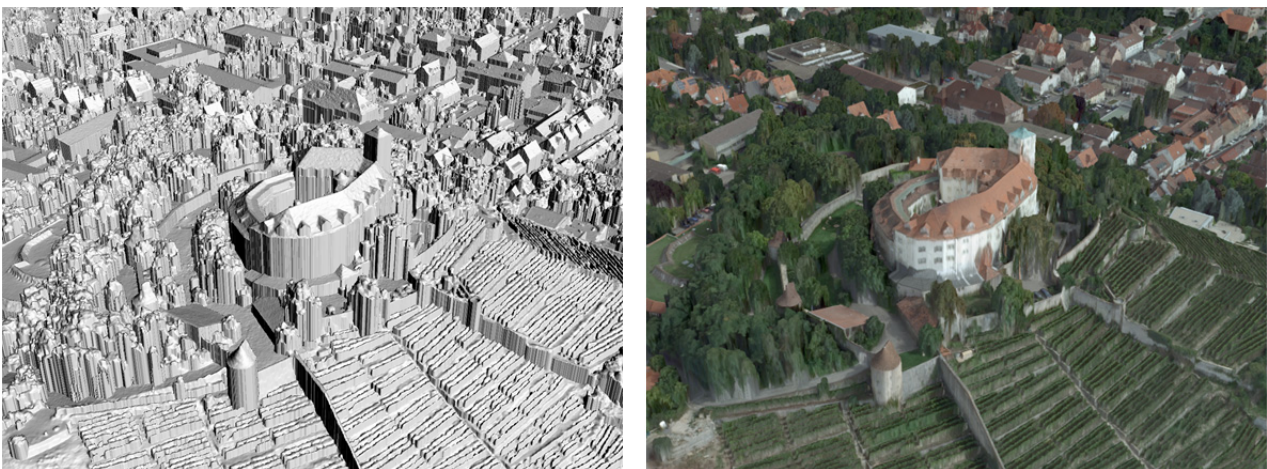
Figure 4: Automatic untextured and textured reconstruction from DGPF UltraCam-X images with 8 cm/pixel ground sampling distance (from Hirschmüller and Bucher, 2010).
