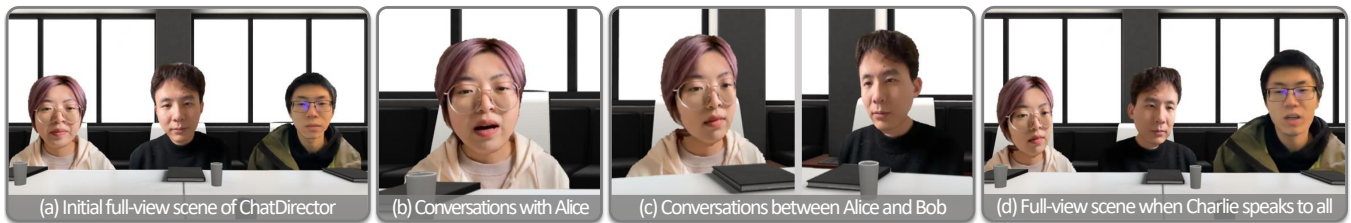
Figure 1: Screenshots of ChatDirector, captured from the local user, Sean’s laptop during a remote meeting with Alice (left), Bob (center), and Charlie (right). (a) Using an off-the-shelf laptop or workstation equipped with an RGB camera, ChatDirector depicts remote participants as 3D portrait avatars and renders them in a shared virtual meeting environment. Sean starts his progress update to the team. (b) When Sean inquires about a feature update from Alice, ChatDirector recognizes the speech activity and automatically focuses the camera on Alice, facilitating a more personal one-on-one discussion. (c) Later, Bob steps in and asks Alice further questions, ChatDirector arranges their avatars in a pairwise layout and simulates direct eye contact by orienting their 3D avatars towards each other. (d) When Charlie updates his progress to everyone, the camera is zoomed out with other avatars turning to Charlie, to provide Sean with a visual cue of the speech transition.
