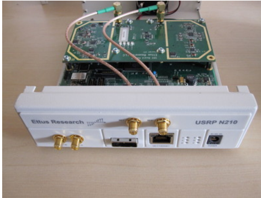
Figure 3.5: USRP without its top cover showing the RF front end and the motherboard under it.
