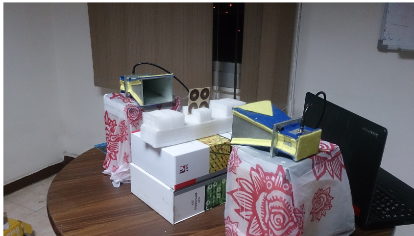
Figure 3.19: USRP test-bed designed to in an indoor office setup.
