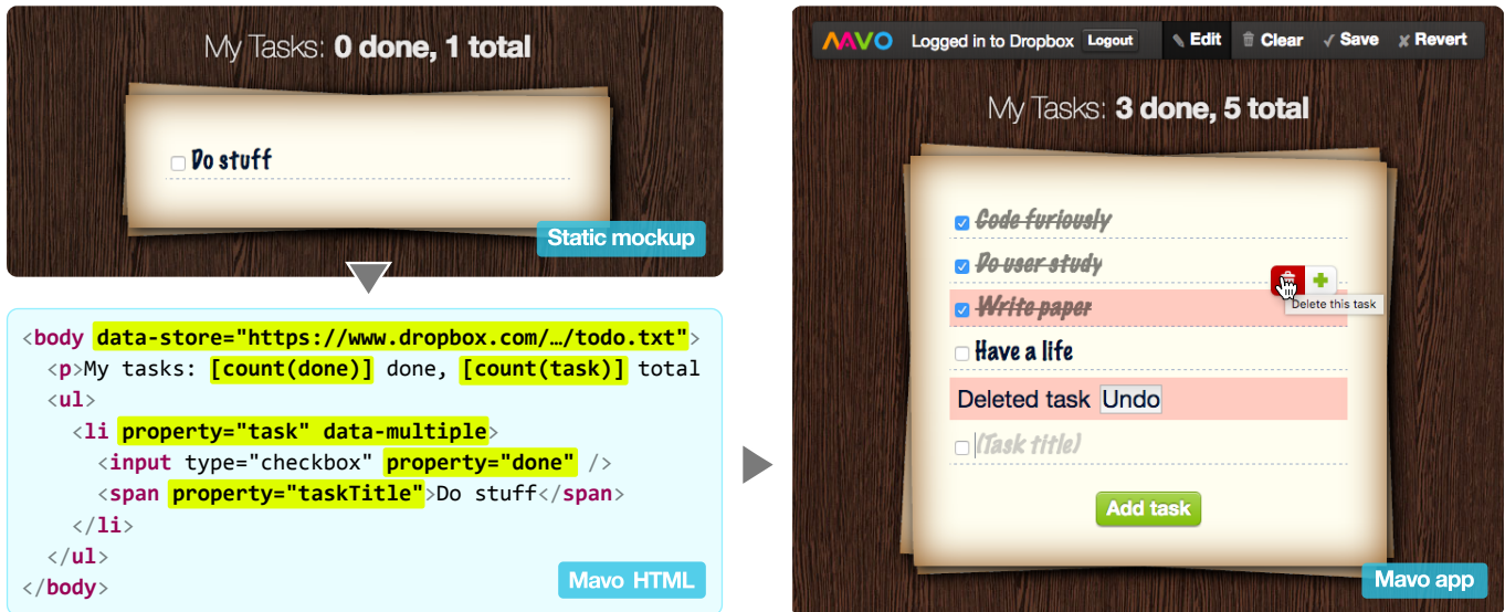
Figure 1: A fully-functional To-Do app made with Mavo, shown with its accompanying code and the starting HTML mockup.
